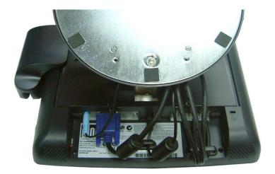
Connect one end of the **customer display cable** to the computer and the other end to the monitor. Secure the cable under the cable management clip.
